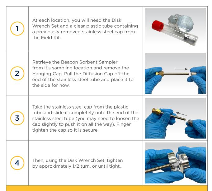
DO NOT OVER-TIGHTEN THE STAINLESS STEEL CAP! Crimping, the end of the tube will prevent a proper seal, damage the tube and potentially ruin the tube. When properly tightened, you should not be able to easily slide the caps off the tube.
